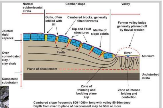
Blocks can back-rotate, forwards rotate or drape the slope
